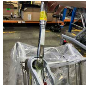
3. Use a torque wrench to tighten the pintle bolt to 25-28Nm
