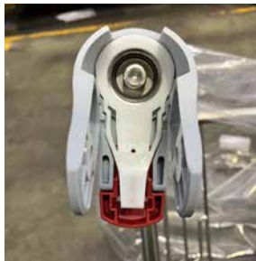
2. End of the pintle bolt is an 8mm hexagonal bolt head
